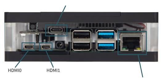
microHDMI - Connection HDMI0 should be used. Especially when 4K resolution is required.
