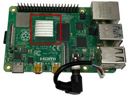
3. Then connect the small board to the two microHMDI connectors and connect the cable from the AUX connector to the board. Make sure that the cable is flat as possible at the board to avoid space problems later.
