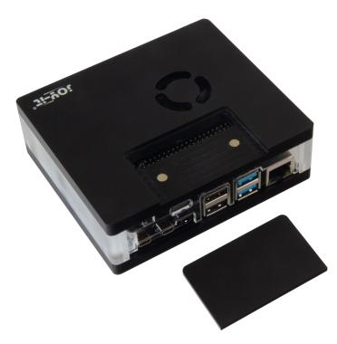
Your case has a removable lid, so the GPIO bar of your Raspberry Pis is still usable despite being in a case.
