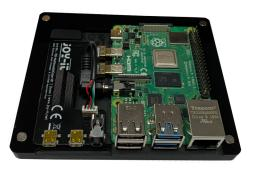
5. In the following step, attach the center piece and push the connection panel into the center piece.
