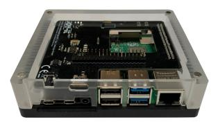
7. Now you have to connect the fan, which is attached at the cover, to the big board. Make sure that the red cable is connected to + and the black cable to -.
