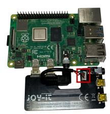
4. Now place the Raspberry Pi with the circuit board on the bottom of the case.
