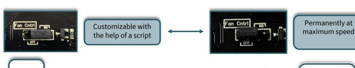
In the provided script a hysteresis is included. This means that if the maximum temperature of 60 °C is exceeded, the system will cool down to the set temperature of 50 °C. Without a hysteresis the cooling would only go below 60 °C.
