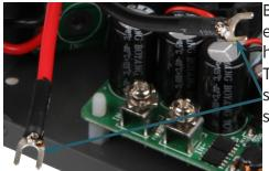
Both sides must be about 5mm at the end stripped because on both ends have to be forked cable lugs attached. These ends should be isolated with shrinking tubes either to prevent shorts. The other end of the cable must be soldered on to the small board.
