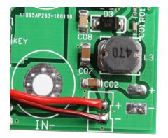
The red cable (+) must be soldered on "+" and the black one (-) on the board at "-".
