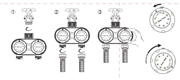
Manual Operation: Rotate dial anti-clockwise to water manually.
