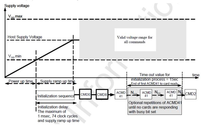
Power up time is defined as voltage rising time from 0 volt to VDD min and depends on application parameters such as the maximum number of SD Cards, the bus length and the characteristic of the power supply unit.
