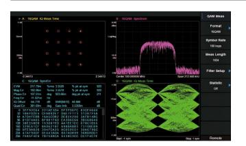
The T3AFG200, T3AFG350 and T3AFG500 optionally supports IQ signal generation with symbol rates between 250 Symbols/s to 37.5 MSymbols/s, providing ASK, PSK, QAM, FSK, MSK and multi-tone signals.
