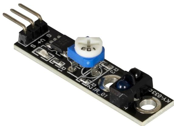
This sensor transmits and receives infrared. It can detect whether it has a reflecting surface (the sensor receives its own signal) or an absorbing surface (the sensor receives no signal) in front of it. You can adjust the sensitivity of the sensor by means of a potentiometer.
