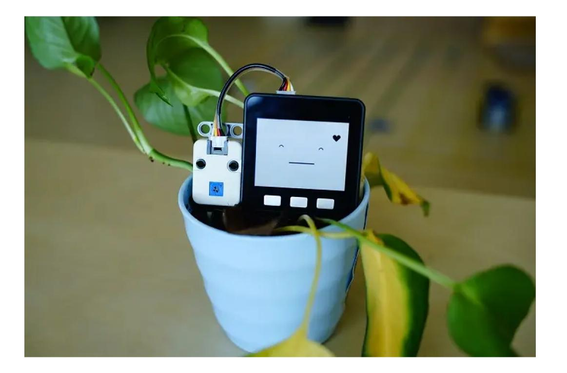
Electrode of the unit is not anti-corrosive, or waterproof, for POC purpose only. Pls do NOT put it in humidity environment for a long while.
