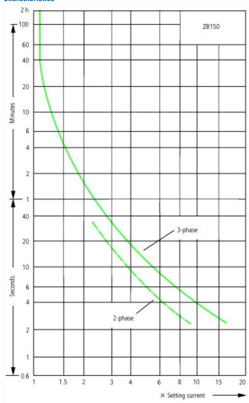
These tripping characteristics are mean values of the spread at 20 °C ambient temperature in a cold state. Tripping time depends on response current.
