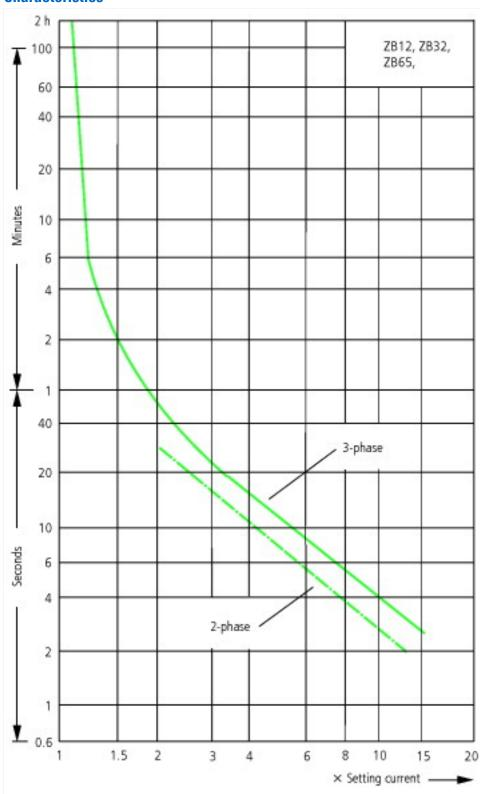
These tripping characteristics are mean values of the spreads at 20  $^{\circ}$ C ambient air temperature in a cold state. Tripping time depends on response current.
