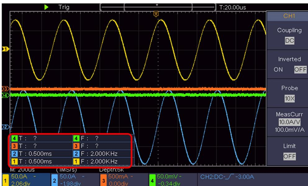
Figure 4- 12 Automatic measurement
