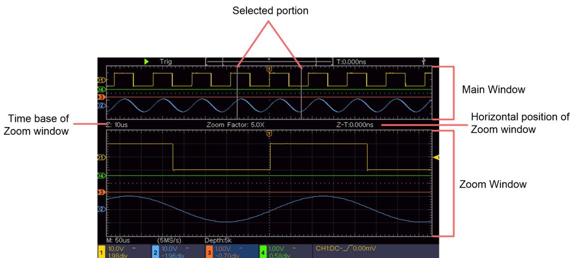
In normal mode, the **Horizontal Position** and **Horizontal Scale** knobs are used to adjust the horizontal position and time base of the Main window.
