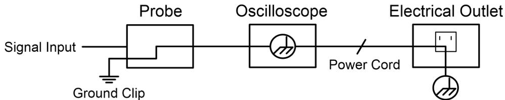
It is not allowed to measure AC power when the AC powered oscilloscope is connected to the AC-powered PC through the ports.
