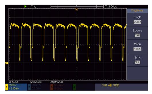
Figure 6-7 Waveform Captured from Video Field Trigger
