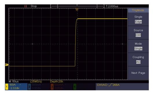
Figure 6-3 Capturing a Single Signal
