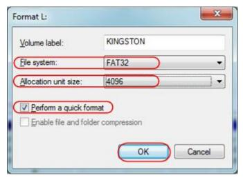
Figure 4-4: Formatting the USB disk setting
