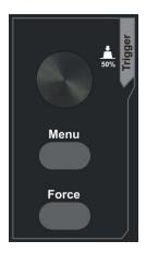
Figure 3-12 Trigger Control Zone
