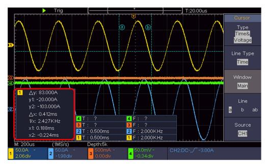
Figure 4-15 Time&Voltage Cursor Measurement
