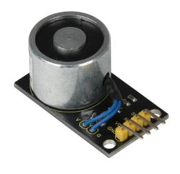
This electromagnet is suitable for smaller projects (e.g. in automation, microcontrollers or robotics). At 5 V, it generates a force of approx. 25 N (approx. 2.5 kg).
