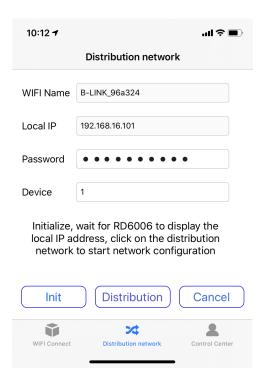
Enter now your password of your network in case that the IP-address on your iPhone is identical with the IP-address of your device. Afterwards, click on *Distribution* to establish the connection.
