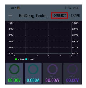
Now you can operate the power supply with your smartphone. Please note, however, that the power supply cannot be adjusted manually as long as your smartphone is connected.
