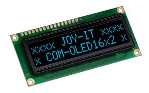
Due to the OLED technology, this display has a high contrast and brightness, as well as a viewing angle of over 175°.
