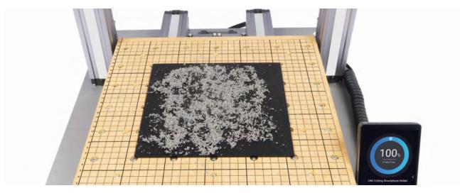
2. Clean the finished work and the machine with a dust collector, and then remove the finished work using the diagonal pliers.
