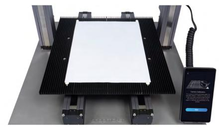
2. Tap Start, and the machine will use the engraved square to calibrate the camera.
