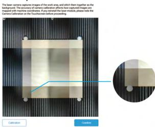
3. ① Open the test file from **Case Library** -> ② Drag the image to where the cutting will take place on the captured platform -> ③ Click **Process** after configuring the settings in **Configurations** section -> ④ Use the default settings specifically configured for the test file -> ⑤ Generate the G-code file -> ⑥ Load G-code to **Workspace** -> ⑦ Set the thickness of the material -> ⑧ Click **Run** .
