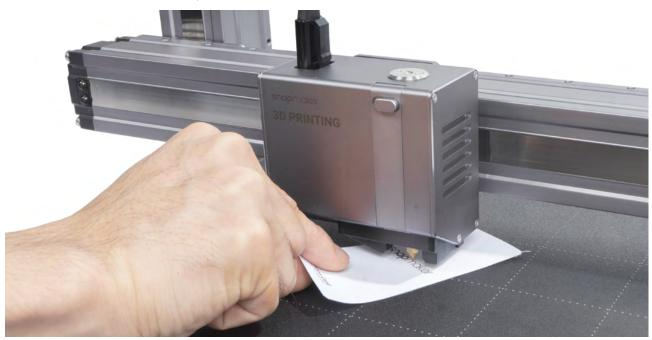
3. Keep adjusting the height of the nozzle using **Up** and **Down** buttons, until you feel slight resistance when you pull out the Calibration Card, and it should be wrinkled when you push it forward. Tap **Save** to save the calibration settings.
