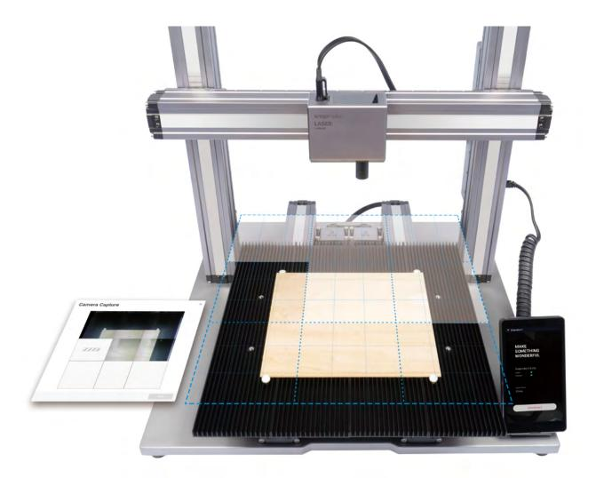
If the edges of the captured image are not aligned, click **Calibration** to manually calibrate the camera.
