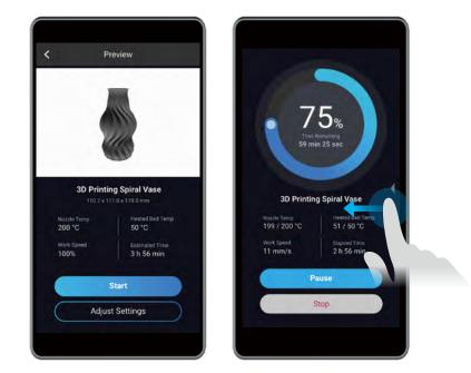
If poor adhesion occurs, swipe left on the printing progress screen and try adjusting the Z Offset. Or you can try leveling the Heated Bed again by selecting **Calibration**. Make sure the tip of the nozzle is clean before you calibrate the bed.
