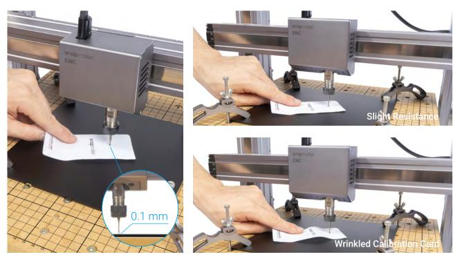
4. Tap **Z+** to lift the CNC Bit until it is above the clamp set, and then tap **Run Boundary** to check if the Work Origin is proper. If any part of the boundary trailed by the CNC Bit goes outside of the material, or if the CNC Bit runs into any portions of the machine, reset the Work Origin and run boundary again.
