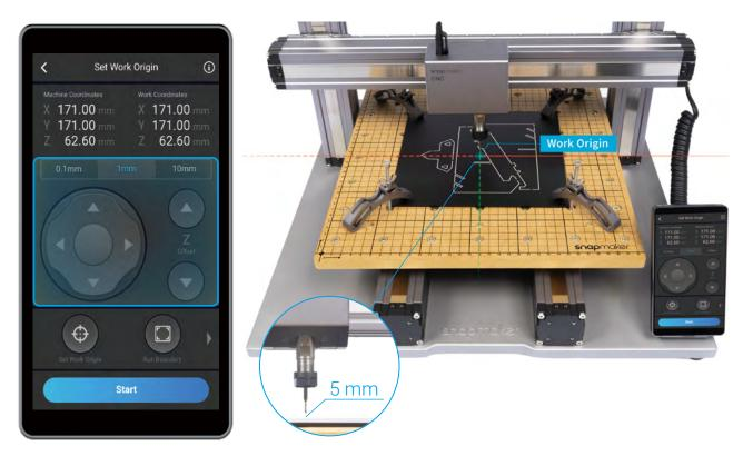
3. Place the Calibration Card or a piece of A4 paper between the CNC Bit and the material. Keep adjusting the height of the CNC Bit using **Z-** or **Z+** buttons until you feel slight resistance when you pull out the Calibration Card, and it should be wrinkled when you push it forward. Tap **Set Work Origin**.
