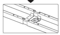
The fixing plate can be attached to either of the right side and the left side.
