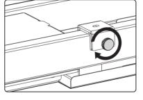
Tighten the knobs on the tray hangers.
