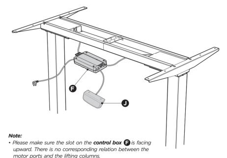
Connect the two motor cords to the two ports marked "M1" and "M2" (one on each side of the
