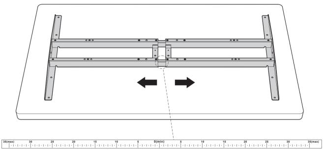
When adjusting the frame position, please make sure it doesn't exceed the range of silk screen printing on the inner crossbar.
