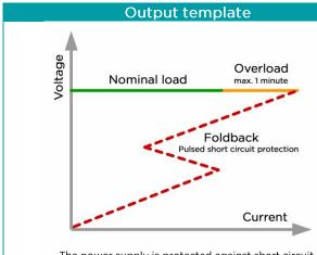
The power supply is protected against short circuit.
