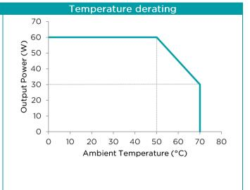
Linear derating from +50°C at 2,5%/°C to 50% load at +70°C
