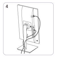
Put both cables in the cable holder on the stand (HOLDER-STAND CABLE) to organise the cables, as shown in the figure.
