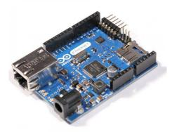
The Arduino Ethernet is a microcontroller board based on the Arduino Uno, and incorporating a WizNet W5100 TCP/IP Embedded Ethernet Controller. It can be programmed like an Uno via a six-pin FTDI -style serial connector. The Arduino <u>USB 2 Serial</u> adapter or any FTDI-style USB-to-serial connector can be used to program it. Additional features coming with the R3 version are:
