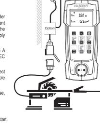
• By pressing the button (7) the automatic test will start.
