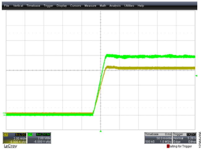
Figure 57. Constant Current Mode in a Load Resistor Green Trace: Output Voltage Yellow Trace: Load Current
