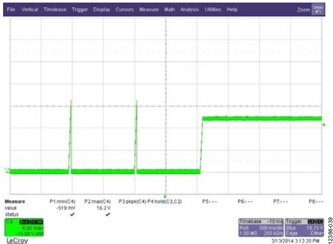
Figure 39. Recovery from VOUT_OV_FAST_FAULT Green Trace: Output Voltage
