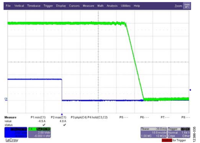
Figure 35. Soft Stop from Light Load Mode Green Trace: Output Voltage Blue Trace: Hardware PSOFF
