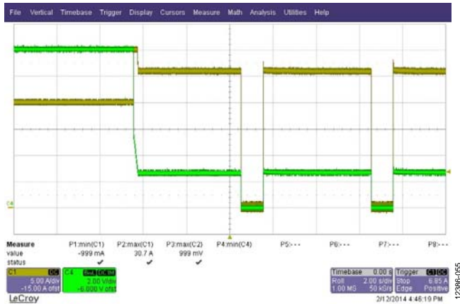
Figure 56. IOUT_OC_FAULT PSU is Set to Enter Constant Current Mode at 27 A. Fault Response Set to Wait for a Debounce of 5 Seconds, Shutdown, and Retry Indefinitely. Green Trace: Output Voltage Yellow Trace: Load Current
