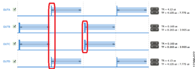
Figure 22. 100 ns Extra On Time Added to OUTB and OUTC
