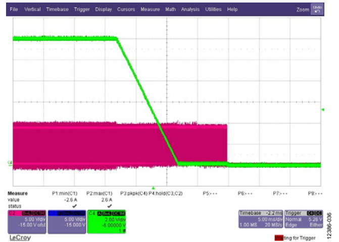
Figure 36. Soft Stop with SR on Time Extension (8 ms) Green Trace: Output Voltage Red Trace: SR1
