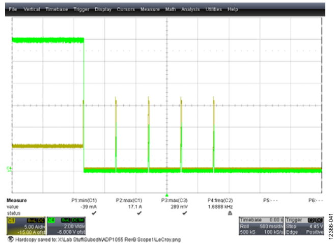
Figure 41. IOUT_OC_FAULT under Short-Circuit Fault Response Set to Shut Down and Retry 4 Times Green Trace: Output Voltage Yellow Trace: Load Current
