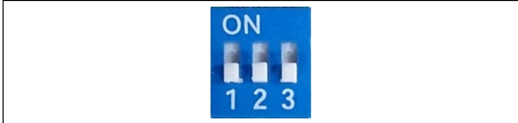
FIGURE 3-1: SW9 IN FLASH APPLICATION MODE
