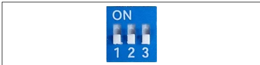
FIGURE 3-35: SWITCH SW9 IN FLASH APPLICATION MODE
