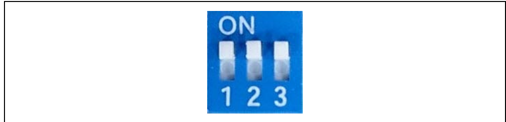
FIGURE 3-36: SWITCH SW9 IN WRITE FLASH MODE
