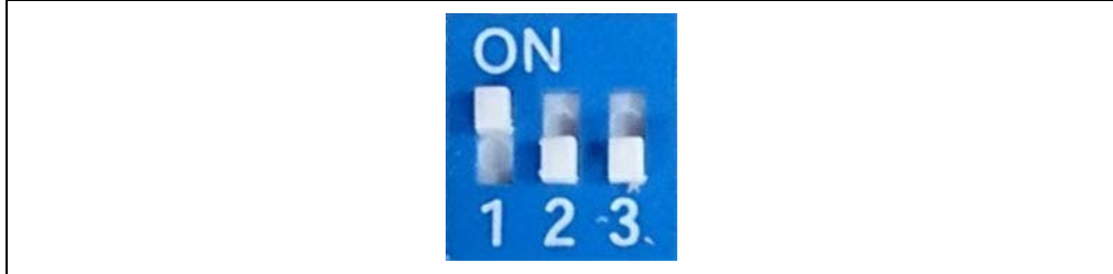
FIGURE 3-29: SWITCH SW9 IN TEST MODE
