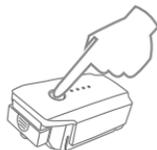
Press the Power Button once Then Press Again and Hold for 2 Seconds to Turn On
