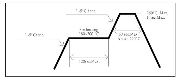
\*Recommended soldering conditions vary according to the type of LED
