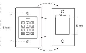
A hole for the connecting cable must be drilled before fastening. Wiring should be carried out according to the wiring diagrams in the following sections.
