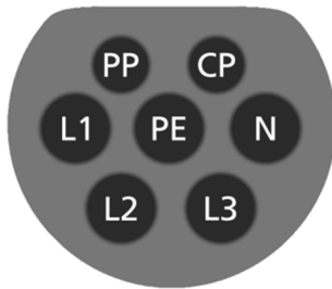
Figure 2: Assignment of the Type 2 connector for connection to the charging station (EVSE)
