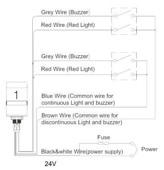
Note: LED wire and buzzer wire can only be connected to one of the common wires.
