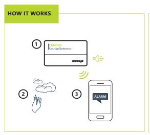
The Mobeye CM4400 smoke detector warns people on the spot in the event of a fire, as well as contacts elsewhere. It makes the difference in helping the vulnerable and in the event of fire in vacant buildings.
