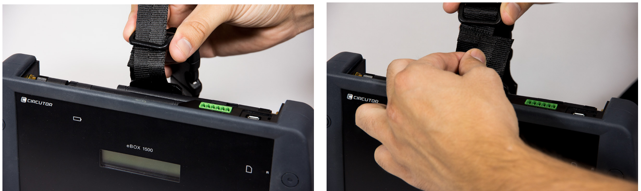
Figure 8: Installation of the fastening strap: Steps 3 and 4.
