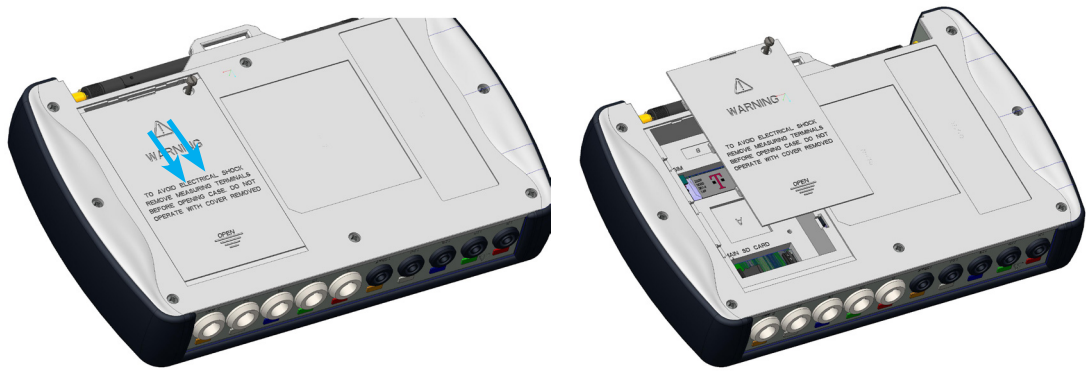
Figure 2:Removal of the battery cover.
