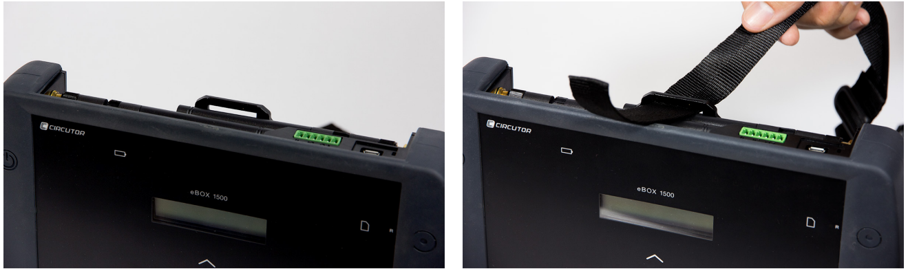
Figure 7: Installation of the fastening strap: Steps 1 and 2.
