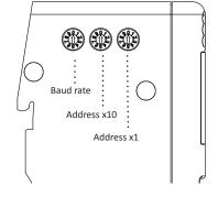
Allowed node address range is 1 - 127. Addresses 1 - 99 are available using the address rotary switches. To set e.g. node address 42, set the left address switch to 4 and the right address switch to 2. Cover the switches with the enclosed switch covers to ensure EMC compliance.
