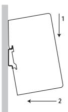
To mount the gateway on a DIN rail, first press it downwards (1) to compress the spring in the rail mechanism, then push it against the rail as to make it snap on (2).
