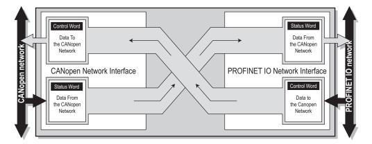
Each buffer holds up to 512 bytes of data, where the first two bytes on the primary network side always are used for control/status information. The remaining 510 bytes gives the theoretical upper limit for the number of data bytes that can be exchanged in each direction. Please note that the actual number of bytes that can be exchanged is highly application and network dependent and can thus be noticably lower than 510 bytes.
