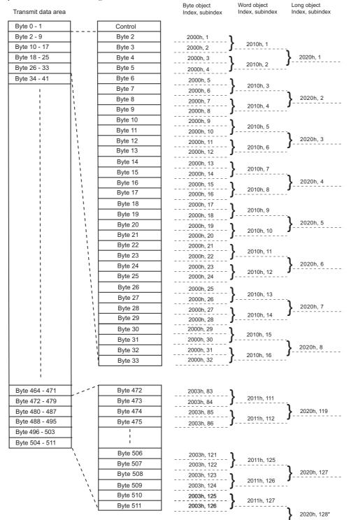
\*The last two bytes are filled up with zeroes
