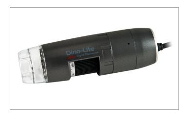
The wide range of magnification (10-140x), the large field of view and working distance of up to 23 cm makes the AM4115TL the ideal solution for all situations where a longer distance between the microscope and the object is required or when it is needed to work under the microscope (repair, rework and assembly tasks etc.)
