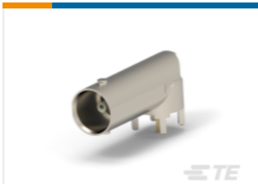
TE Part #5413558-3 BNC RF Connector: Male (Jack), Right-angle, 75 Ohm, 2 Ghz
