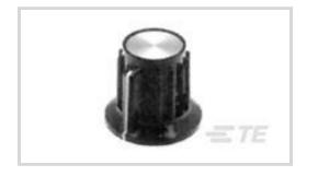
Switch Knob Product Type: Knob Switch Knob Material: Phenolic Knob Design: Ribbed with Bar Pointer Shaft Size: 6.35 mm [.25 in] Switch Knob Diameter: 24.8 mm [.976 in]
