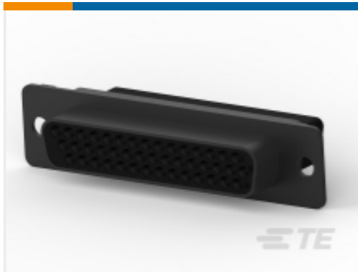
TE Part #1658683-1 D-Sub Crimp Recept Signal 44 Posn, Socket Size 22, Shell Size 3
