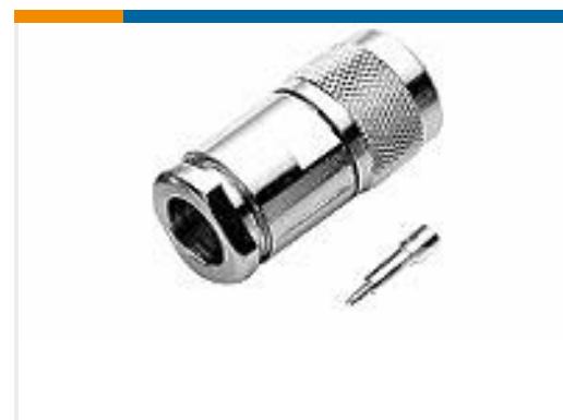
TE Part #1-1478419-0 N Str Plg PS 50Ohm Silver Pltd RG58C /U,
