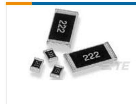
TE Part #1623516-1 CRG1206 1% 470K
