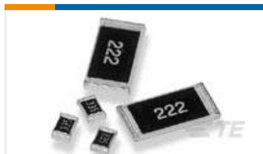
TE Part #2-1879502-8 CRGH2512 5% 180K 2W
