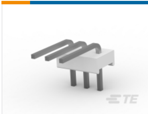
TE Part #1-640457-3 Polyester Right Angle PCB Header: 2.54mm, Unshrouded, MTA 100
