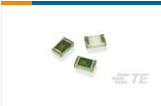
TE Part #1-1879133-9 RN 0603 1K27 0.1% 10PPM 1K RL
