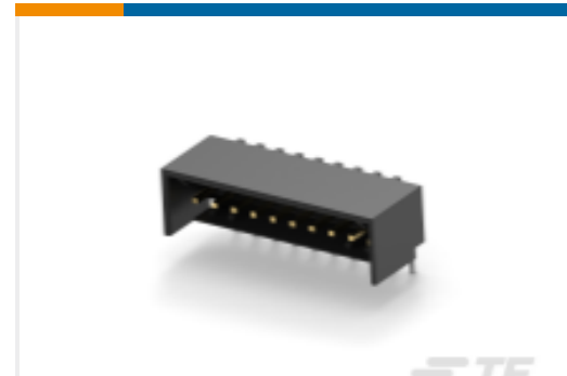
TE Part #2-644488-6 Polyester Right Angle PCB Header: 2.54mm, Shrouded, With Mating Alignment
