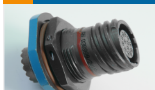
TE Part #YDTS24Z15-97PNV001 Jam Nut: D38999, 15-97 Insert, Black Zinc Nickel Plating
