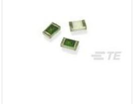
TE Part #1676678-2 RN 0805 27R4 0.1% 10PPM 1K RL
