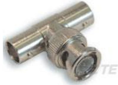
TE Part # 6-1337458-0 BNC T Adpt JPJ 50Ohm Nickel Gold Pltd
