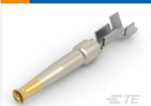
TE Part #1658543-2 D-Sub Conn Contacts: Socket, Phosphor Bronze, Signal, Size 20
