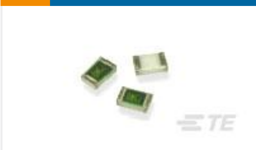
TE Part #1676359-2 RN 0805 4K53 0.1% 10PPM 1KRL
