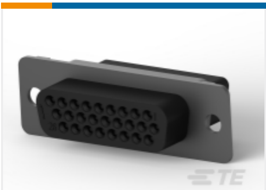
TE Part #1658687-1 D-Sub Crimp Recpt Signal 26 Posn, Socket Size 22, Shell Size 2
