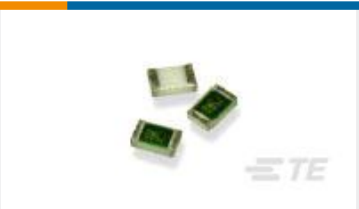
TE Part #1879217-3 CPF 0603 160K 0.1% 25PPM 1K RL
