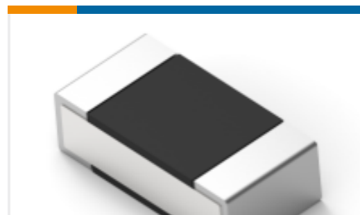
TE Part #1-2176308-6 RP 1E 0.1W 191K 0.1% 25PPM 5K RL
